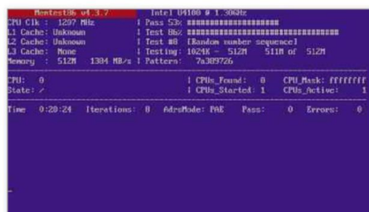
Resolve blue-screen error messages on your laptop by fully inserting its modules or using the MemTest86 tool
